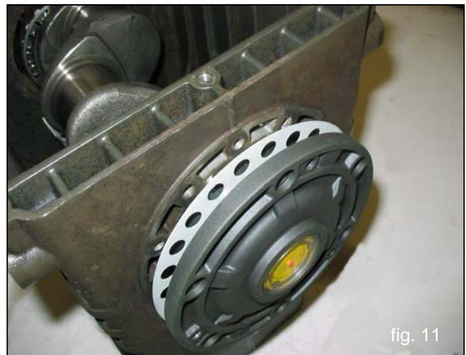
E) Insert the shims under the cover on the sight glass side (see fig. 11), fixing it to the crankcase using the appropriate screws, and verifying that the stall torque is between 4 Nm and 7 Nm.
