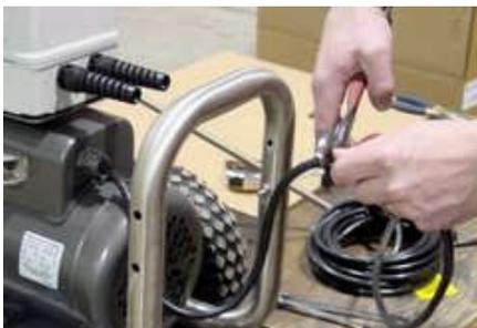
3. Cut the power cord at 21" from motor strain relief.
