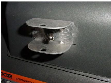
11. Ensure that the motor switch is in the ON position
