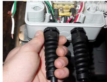
5. Insert the motor cord into the box through the left side strain relief and hand tighten.
