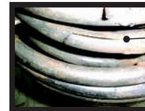
This is an example of a coil that has split due to freezing. The tell-tail sign is a split in a horizontal direction.
