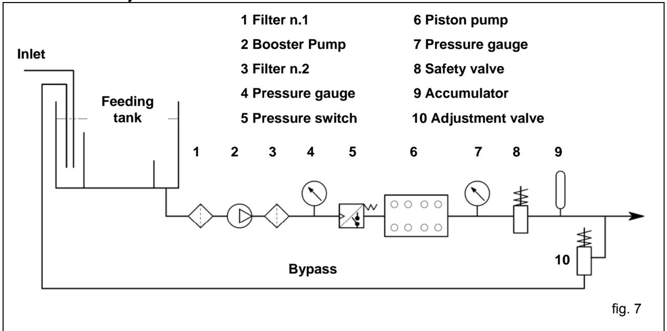
**With the pneumatic adjustment valve.**
