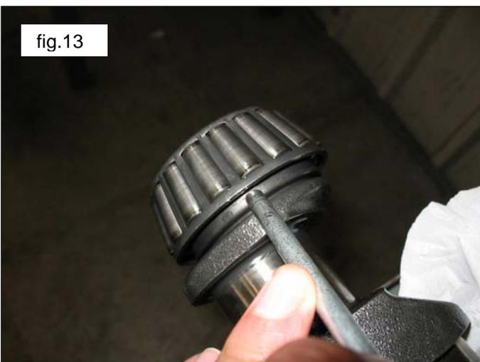
The new bearings can be mounted cold with a press or rocker, supporting it on the lateral surface of the ring nuts involved in press fitting with the rings. The press fitting operation can be facilitated by heating the involved parts to a temperature between 120° - 50° ( 250° - 300° ), ensuring that the ring nuts go down to end stroke in their seats.
