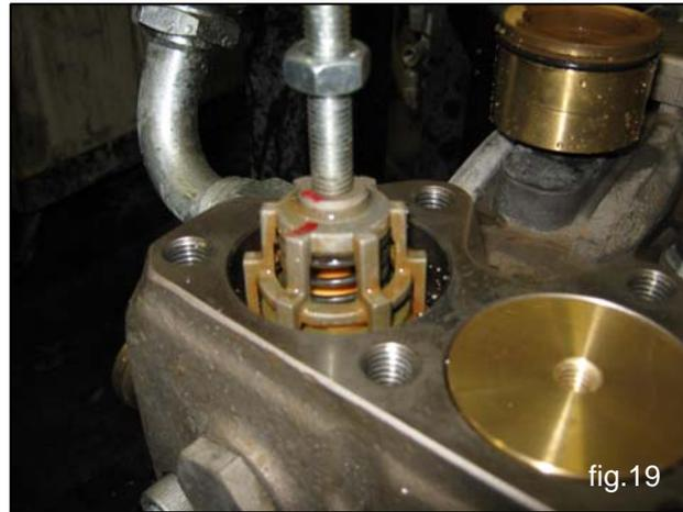
Dismantling of the suction and outlet valve units can be carried out screwing in a sufficiently long M10 screw which can move the valve plate and remove the valve guide from the seat ( fig. 20) ; pos.1 . If the threaded holes should not be present on the valve guides, dismantling can be easily carried out by leveringaging with simple tools fig. 21.
