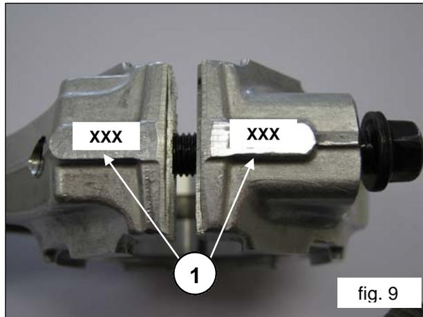
Fasten the caps to their respective con-rod shanks by means of M8x1x42 screws (fig. 10) lubricating both the underhead and the threaded shank, proceeding in two different stages:
