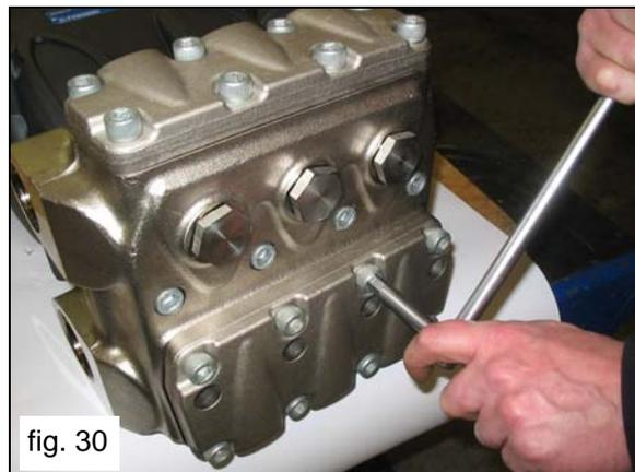
Extract the valve plugs using a slide hammer cod. 26019400 combined with the tool cod. 27513600 (fig.31).
