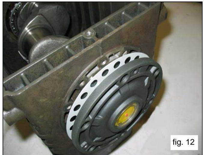
Insert the shims under the cover on the sight glass side (see fig. 12), fixing it to the crankcase using the appropriate screws, and verifying that the stall torque is between 4 Nm and 7 Nm.
