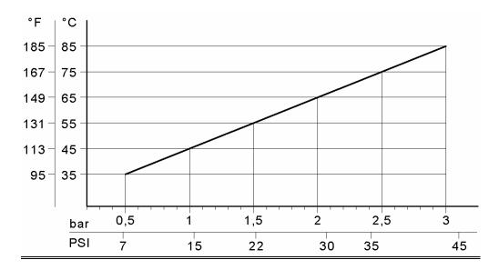
Naturally, if the application allows to feed the pump with 45 PSI even at low temperatures (for example: 115°F) the life of the wet end of the pump will be even longer.
