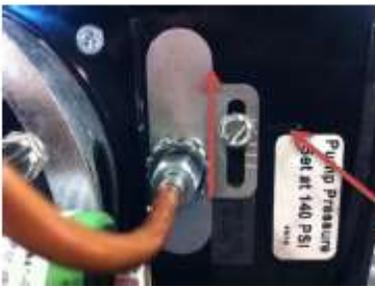
MOVE ELECTRODE ASSEMBLY DOWN BY PULLING GENTLY ON COPPER TUBE NUT. THIS MOVEMENT WILL REPOSITION THE INDICATING LINE UP ONE NOTCH ON THE ADJUSTER PLATE. TIGHTEN NUTS.
