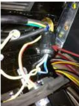
CLIP FERRITE AROUND THE THREE IGNITER WIRES AS CLOSE TO THE IGNITER BODY (WIRE COLOURS BLUE/WHITE, BLACK, WHITE). CLOSE ASSEMBLY AND TIGHTEN.
