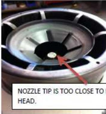
NOZZLE TIP IS TOO CLOSE TO BURNER HEAD.
