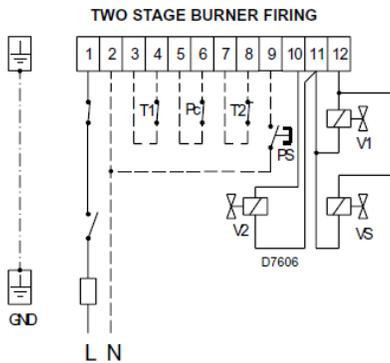
**Note:** If an external electrical source is utilized, the conversion burner, when installed, must be electrically grounded with a solid green wire to Earth Ground, in accordance with local codes or, in the absence of local codes, with the National Electrical Code ANSI/NFPA 70-1990 and the CSA Electrical Code.
