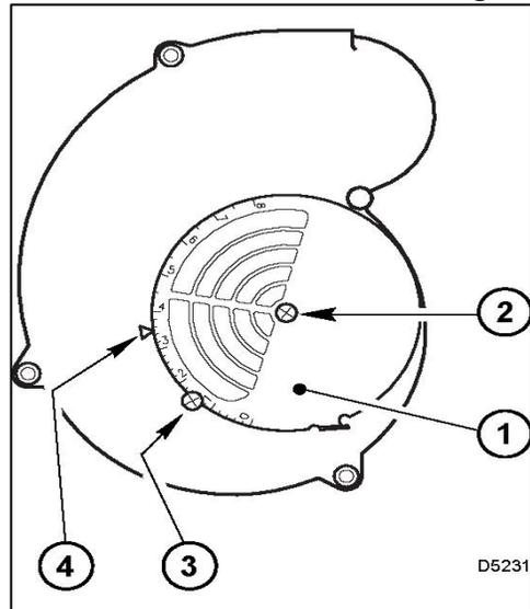
**NOTE:** Variations in flue gas, CO<sub>2</sub> and temperature readings may be experienced when the burner cover is put in place. Therefore, the burner cover **must** be in place when making the final combustion instrument readings, to ensure proper test results.
