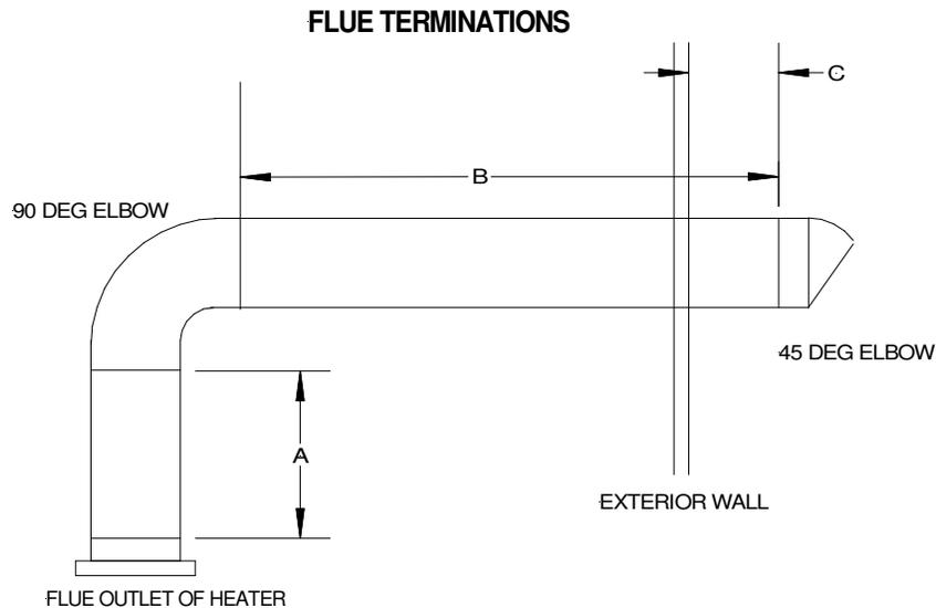
A - Vertical vent run must be a minimum of 2ft from heater outlet.
