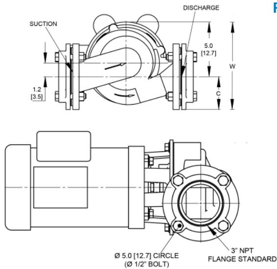
**PUMPS ARE DESIGNED TO MOUNT HORIZONTALLY OR VERTICALLY**
